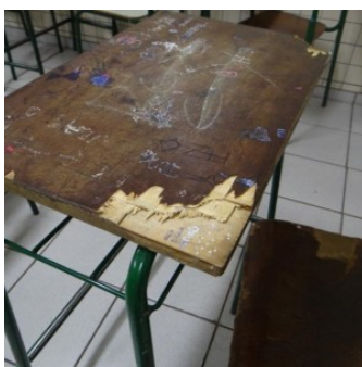
[Figure 01] Deteriorated laminated material used in school portfolio (Source: http://ecoeducar.com.br )
