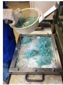
[Figure 06] Recycled aggregate blend + polyurethane vegetable resin + glass fibers (Source: Baldan, 2015)
