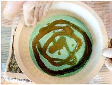
[Figure 05] Recycled aggregate + polyurethane vegetable resin (Source: Baldan, 2015)
