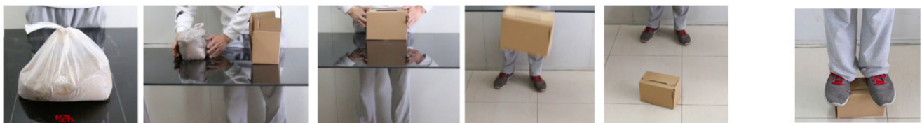
[Figure 7] Load bearing strength test. [Figure 8] Compression strength test of new express packaging structure
