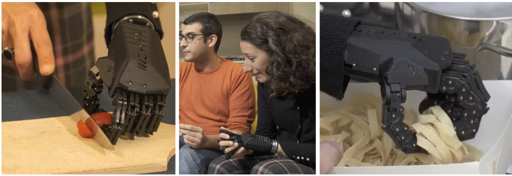
[Figure 1] The SoftHand adaptable and gentle grasp. In the middle, its self-interactions feature exploited.
