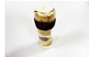
[Figure 3] Frugal thermos made with insulating materials - saw dust and coffee powder
