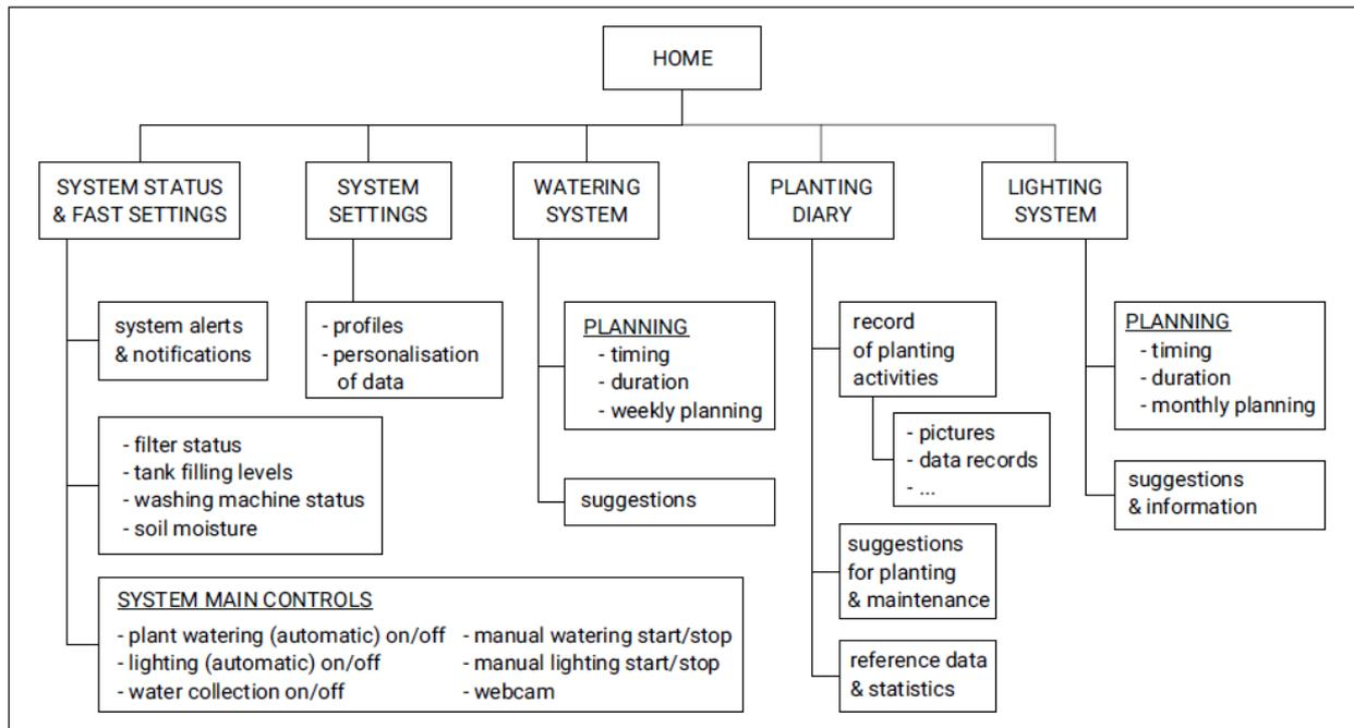
[Figure 3] Workflow of the final user interface for system control
