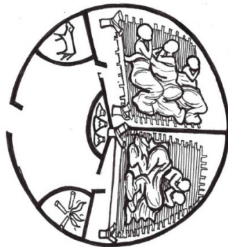
Figure 2 Kinyankole house lay out showing the bedrooms, platform for milk containers, fire place and place for newly born calves (illustration by Banga Simon)
