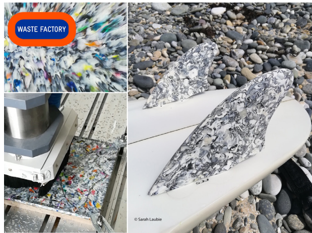
[Figure 4] Recycled Surf fins developed in the Waste Factory project © Sarah Laubie
