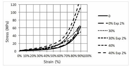
[Figure 6] Representative stress-strain curves obtained by mechanical compression test performed on the Water shaped disks made with different PVA:MCC Poly-Paper ratios expanded and non-expanded.
