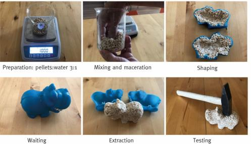
[Figure 2] Water Shaping process stages
