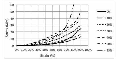
[Figure 5] Representative stress-strain curves obtained by mechanical compression tests performed on the Water shaped disks made with different PVA:MCC ratios.
