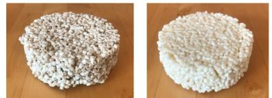
[Figure 4] Discs obtained by Water Shaping process (diameter =101 mm, beight = 36 mm). On the left: 70:30 PVA:MCC disk without expander; on the right: a disk obtained with the same PVA:MCC ratio, additioned with the expanding agent.
