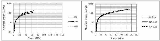
[Figure 7] Representative stress-absorbed energy of the Water shaped disks made with different PVA:MCC Poly-Paper ratios non-expanded (left) and expanded (right).
